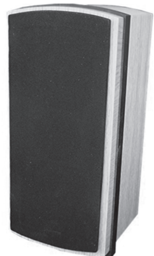
PHOTO 5: Completed cab with grille.
