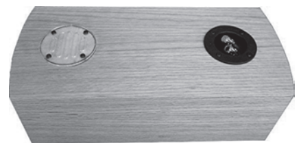
PHOTO 4: Installed input cup and aperiodic vent.
