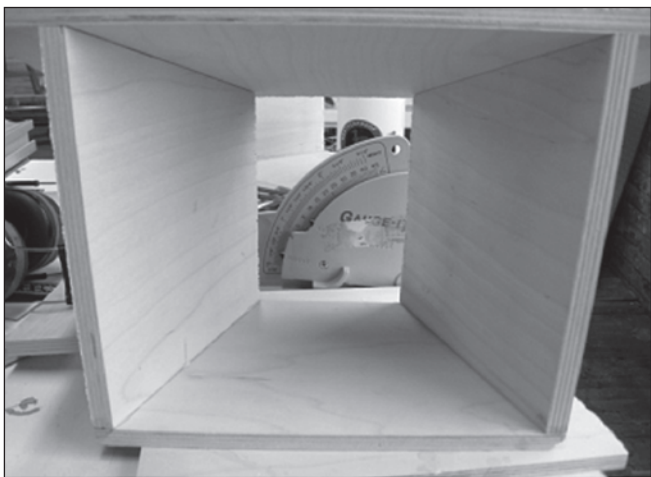
PHOTO 5: After the cut, the top piece now fits tight to the side pieces.
