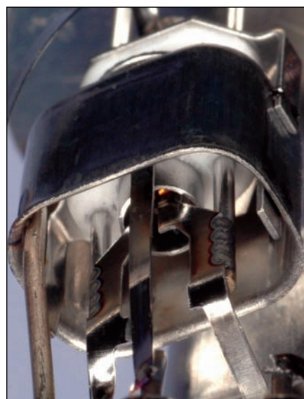
PHOTO 4: Close-up of cathode assembly.
