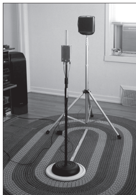
PHOTO 1: Auratone 5C Super Sound Cube loudspeaker mounted on top of a tripod-style mike stand. Dipole microphone prototype is supported by a mike stand sitting on a cheap turntable. Speaker and microphone are positioned 1m apart, midway between floor and ceiling, near the middle of the room.
