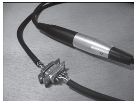
PHOTO 2: Closeup of computer connectors wired in star-quad configuration. This connector pair is inserted in the middle of a star-quad mike cable, which was made by cutting the ends off a shielded MIDI cable and installing XLR connectors.
