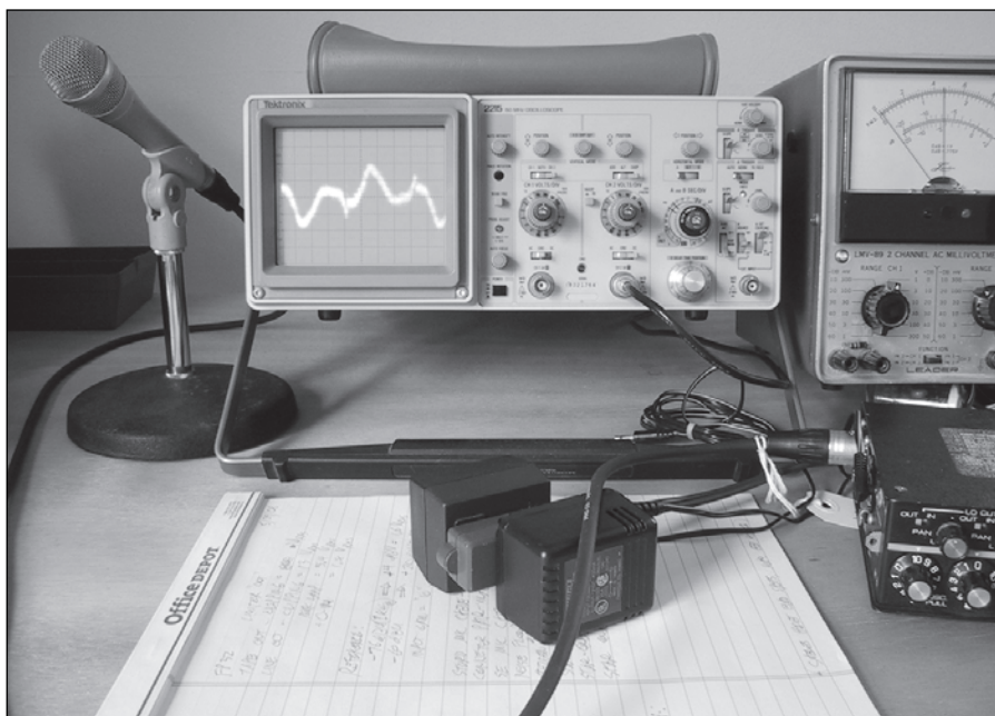
PHOTO 1: Bench setup for measuring induced hum. Note that instruments have been pulled together for the snapshot, but were farther apart for actual measurements. This was necessary because each instrument has its own power transformer and stray magnetic field. Microphone shown was replaced with a shorted plug for actual measurements.
