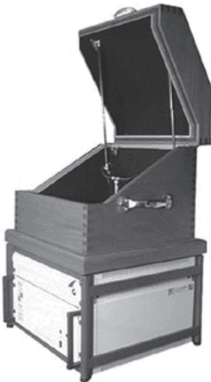
PHOTO 2: Microphone Calibration Workstation, model 9350C from the Modal Shop, Inc., www.modalshop.com . When the lid is closed, some sound isolation is provided for the microphone calibration.
