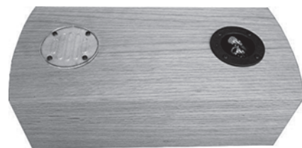
PHOTO 4: Installed input cup and aperiodic vent.
