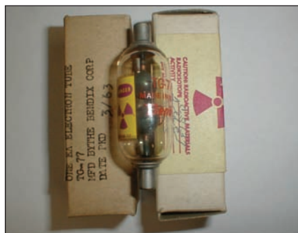
PHOTO 2: The Bendix TG-77 radioactive tube.
