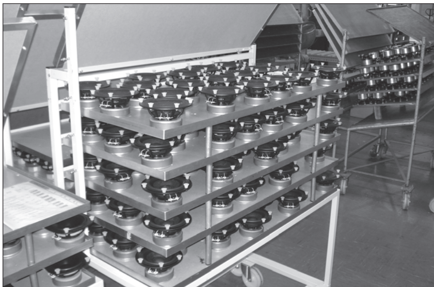
PHOTO 7: Completed drivers waiting for final QC test before being shipped.
