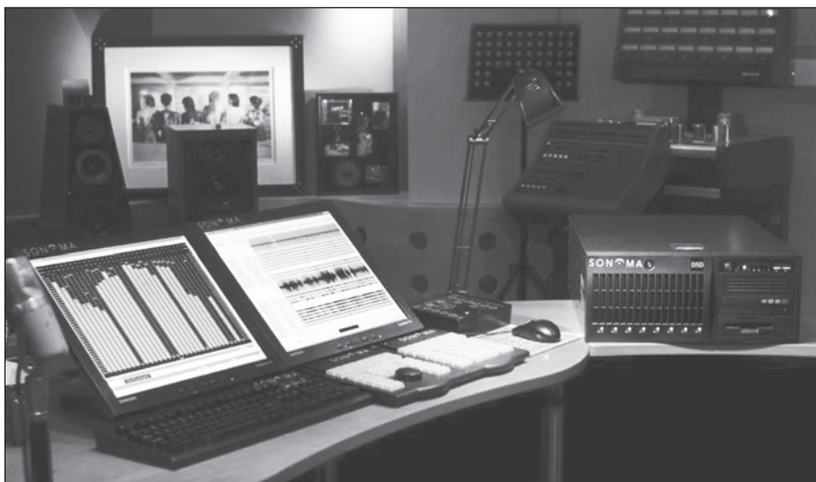
PHOTO 1: Sonoma’s DSD-Pure multi-track recording and editing system operates entirely in the DSD domain. Leading recording engineers and producers have proclaimed it the most transparent recording and editing system available. (Courtesy of Super Audio Center, LLC)
