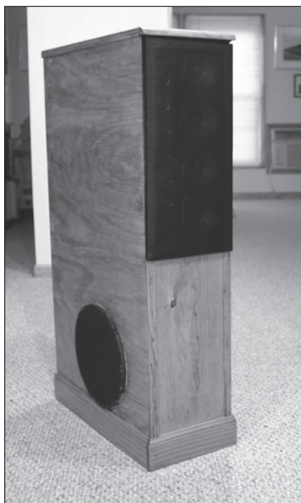
PHOTO 7: Finished enclosure with grille.
