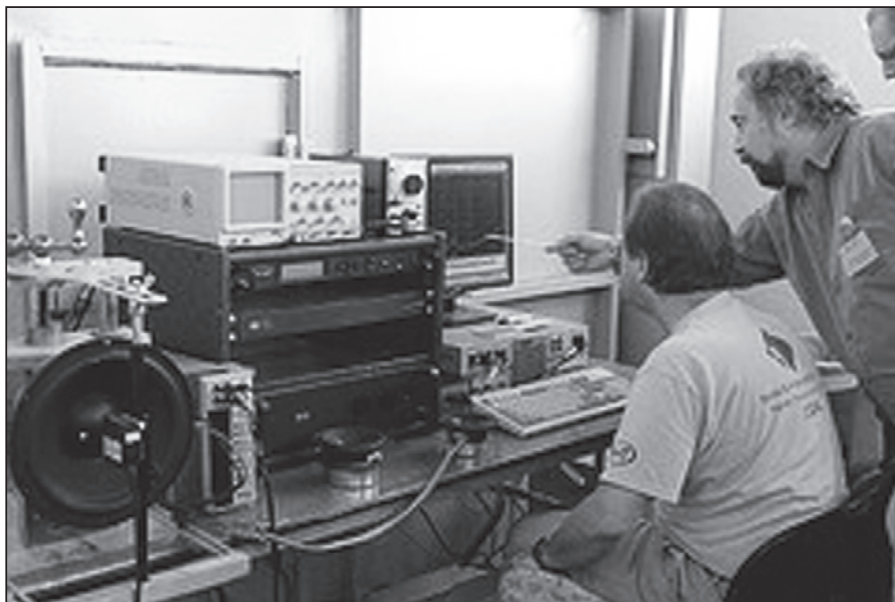
PHOTO 5: Klippel driver measurement system.
