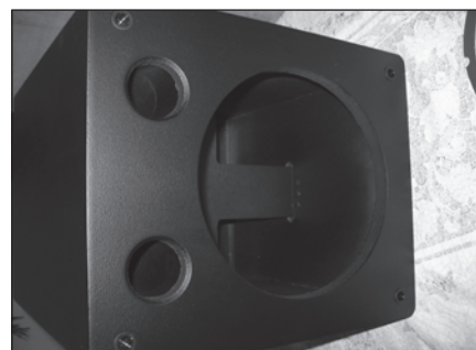
PHOTO 4: The front of the MDF cabinet, showing the woofer opening and two ports.
