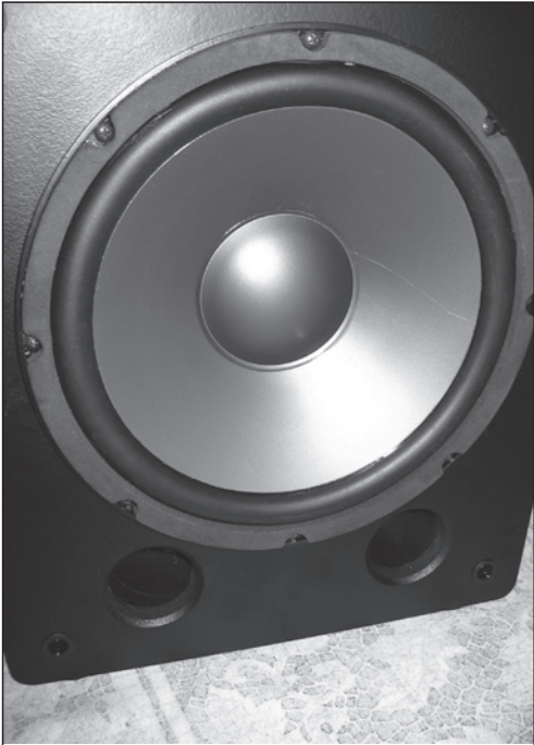
PHOTO 10: The woofer mounted in the cabinet.
