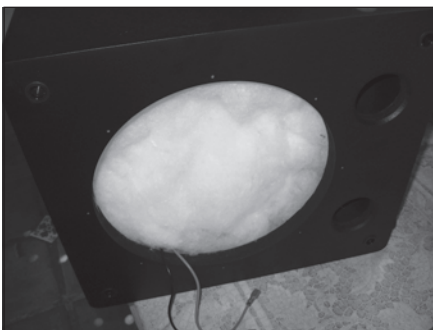
PHOTO 8: The fully stuffed cabinet, ready for mounting the woofer.
