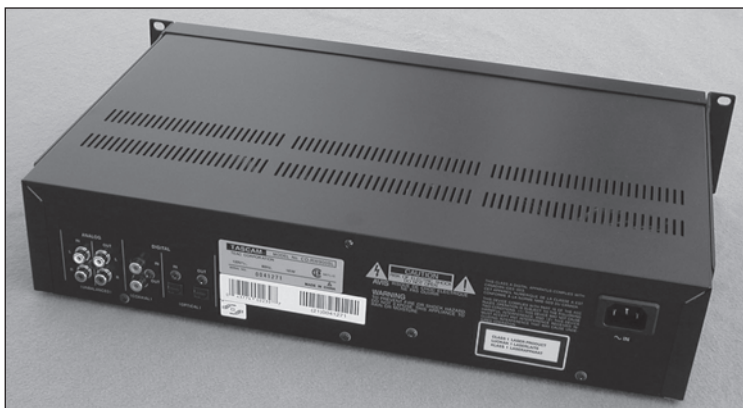
PHOTO 2: Rear view of the Tascam CD recorder. The CD-RW900SL has unbalanced analog inputs and outputs, plus S/PDIF and Toslink Optical digital I/O. The CD-RW901SL version adds balanced analog connection, plus AES/EBU digital I/O.
