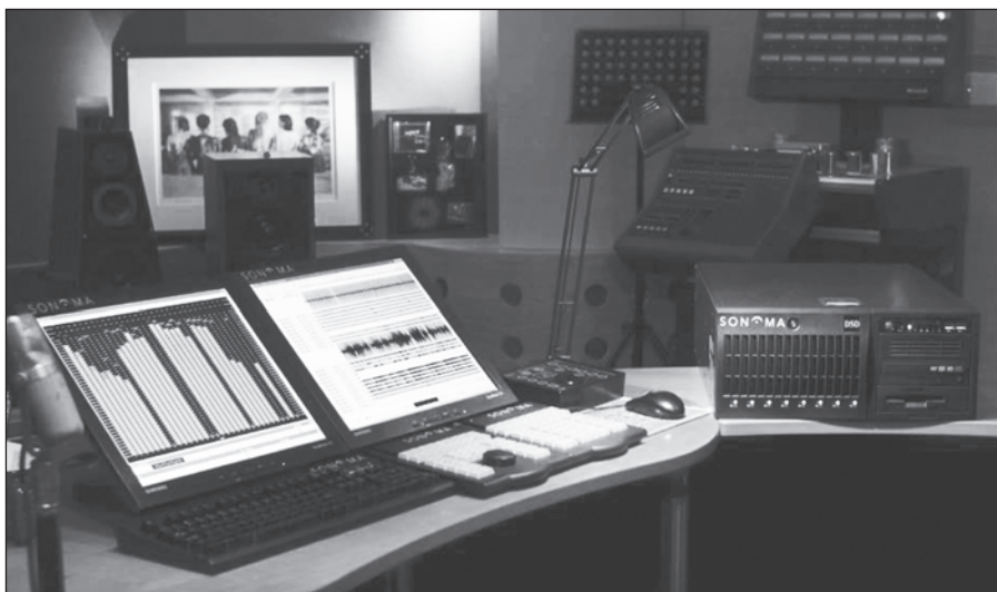
PHOTO 1: Sonoma's DSD-Pure multi-track recording and editing system operates entirely in the DSD domain. Leading recording engineers and producers have proclaimed it the most transparent recording and editing system available. (Courtesy of Super Audio Center, LLC)
