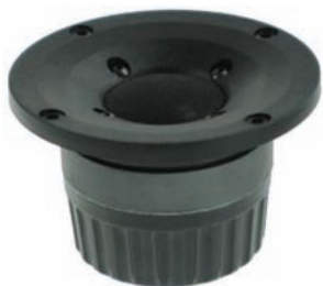
PHOTO 4: The concave and angled surfaces of the DXT driver prevent beaming at higher frequencies.
