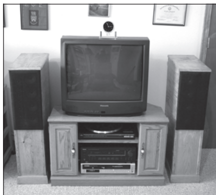
PHOTO 8: Finished enclosure pair.
