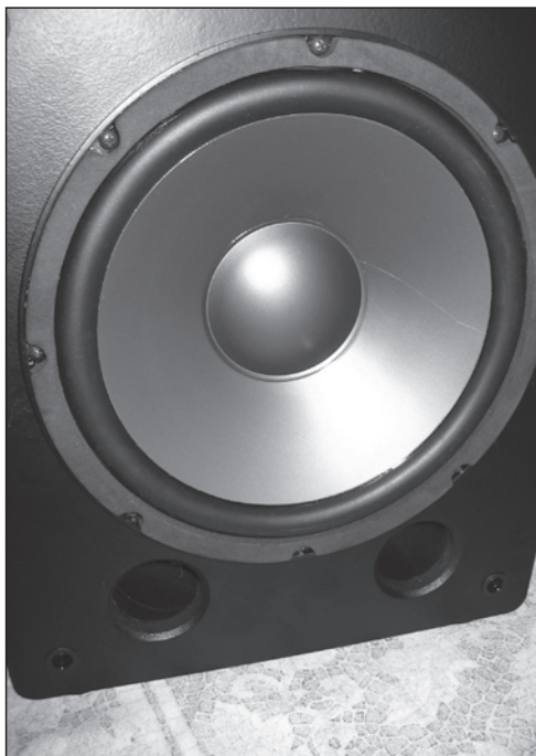
PHOTO 10: The woofer mounted in the cabinet.
