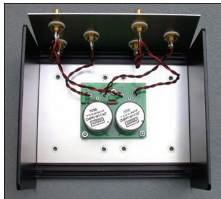
PHOTO 3: Jensen CI-2RR, audiophile version. The Jensen PC board is mounted in the Wolfram MC-5A enclosure. Vishay/Dale RN60 metal film resistors and Wima FKP2 polypropylene capacitors replace the R/C components supplied by Jensen.
