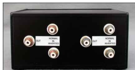
PHOTO 2: Rear panel of the transformer enclosure, showing DH Labs' excellent CM-R1 chassis-mount RCA jacks. Normal and reverse-polarity inputs are included.
