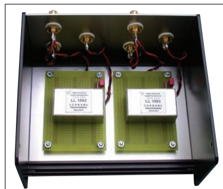
PHOTO 1: A pair of Lundahl LL1592 line input transformers mounted on Old Colony D-4 prototyping boards in a Wolgram MC-5A enclosure with gold-plated, Teflon-insulated connectors.
