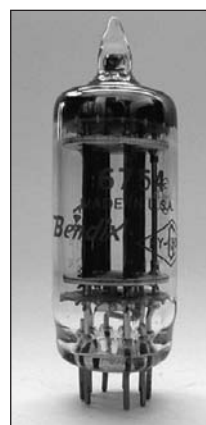
PHOTO 1: 6754 TE-36 miniature tube tip-off.
