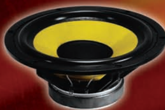
S05-181-V3 8" CAST FRAME WOOFER, 28 OZ MAGNET, WOVEN FIBERGLASS CONE BUTYL RUBBER EDGE
