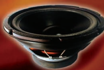
OC10W-8B 10" WOOFER, 40 OZ MAGNET, 2" V.C. POLYPROPYLENE CONE WITH POLYETHER FOAM EDGE
