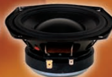
SMB-50 5.25" MID-WOOFER SANTOPRENE EDGE VENTED POLE
