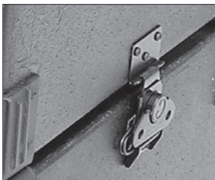
PHOTO 6: Latching cabs together.
