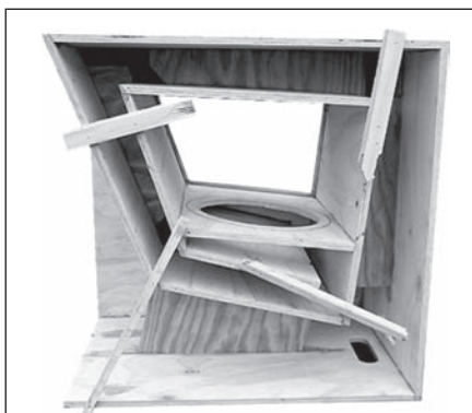
PHOTO 4: Temporary braces keep panels squared.
