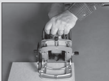
PHOTO 10: Slots cut into faceplates.
