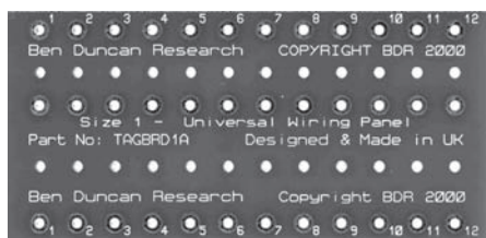
PHOTO 5: Ben Duncan's TAGBRD1A Tag Board is designed for point-to-point wiring, particularly tube circuits. The board is made of durable green fiberglass and rugged, plated-through holes.
