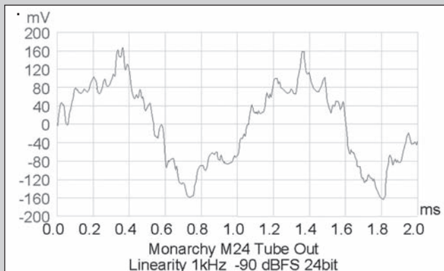
FIGURE 7: 1kHz undithered sine wave -90.3dBfs tube Dac output (24 bit data).
