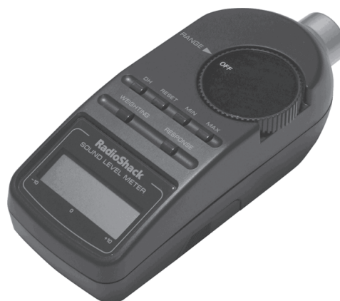
PHOTO 3: RS digital-display sound level meter.
