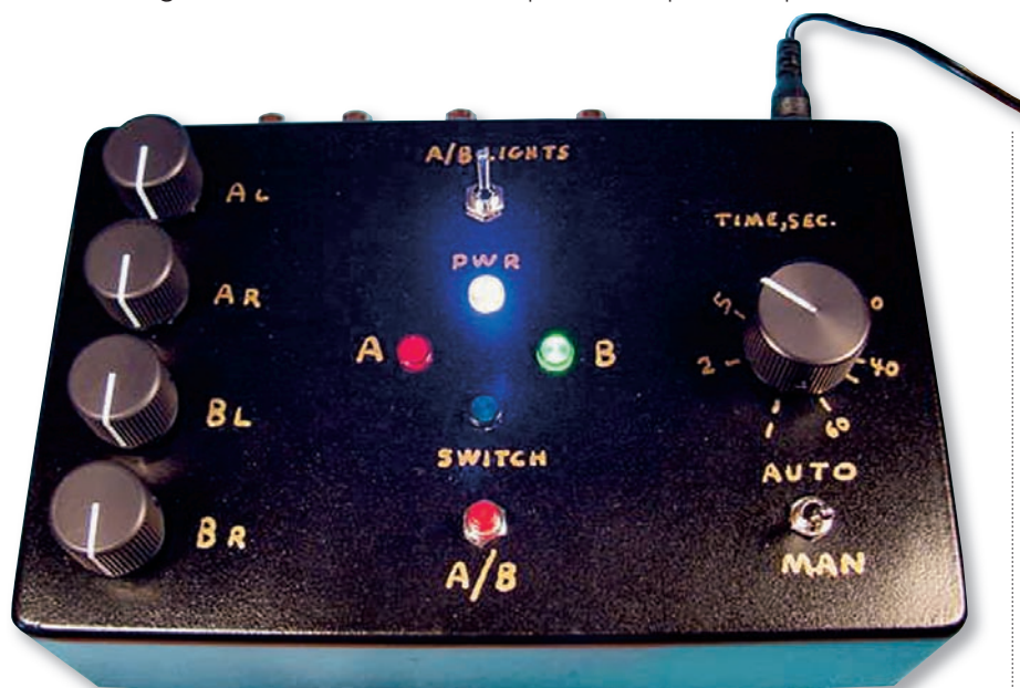
PHOTO 1: Switch box for testing.
