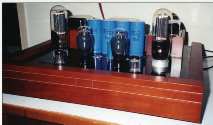
PHOTO 2: Stereo 2 x 40W power amp using 211 outputs driven by 6L6 in triode mode, plus 6SN7 inputs and an interstage transformer.
