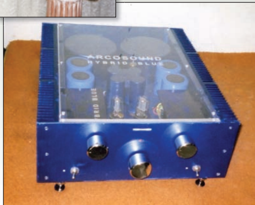
PHOTO 4: A hybrid two-channel, 240W amplifier with an integral tube pre-amp.
