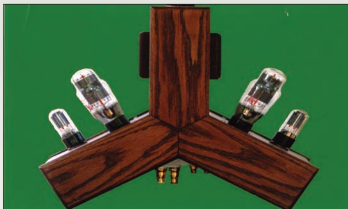
PHOTO 1: Single-ended, stereo 3.5W/channel using 2A3s for output, driven by 6SL7s.
