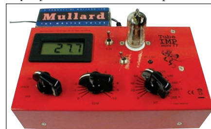
PHOTO 2: Tube Imp testing Mullard ECC83.
