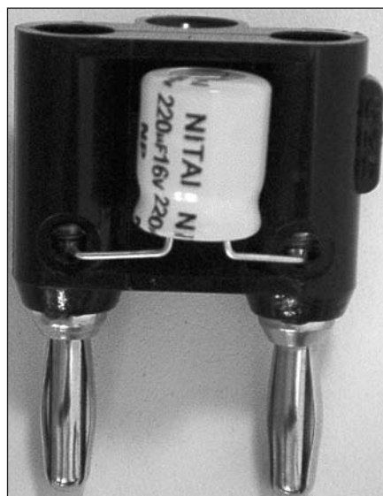
PHOTO 1: A capacitor mounted on a dual banana plug.
