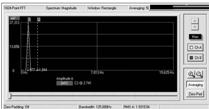
FIGURE 4: Distortion components of a 1kHz signal at 50W into 8Ω (54V pp).
