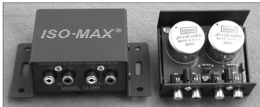
PHOTO 2: Jensen's Iso-Max CI-2RR transformer-coupled stereo audio ground isolator is ideal for interfacing audio and video systems. The transformers are among the world's finest, with very transparent sonics.
