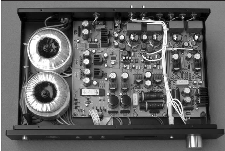
PHOTO 3: Inside the M24. Two power transformers are used, one for analog and the other for digital circuitry. Construction is robust and parts quality is high, with Teflon-insulated internal audio wiring.
