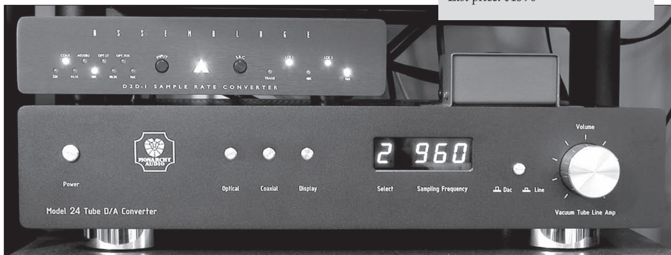
PHOTO 1: Monarchy M24 DAC in one of my equipment racks. Sitting on top is the Parts Connexion D2D-1 Sample Rate Converter and the Jensen IsoMax CI-2RR. The M24 features a robust steel chassis, and a thick, brushed, and anodized aluminum front panel with rounded corners, making a nice visual match for the D2D-1. Monarchy's DIP Upsampler and GW Labs' DSP Upsampler should also work well with the M24.
