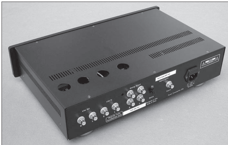
PHOTO 2: M24 rear panel. From left to right, the pair of Line Outputs from the tube line amplifier, Line Inputs to the tube line amp, and the DAC outputs, tube on the bottom and solid-state I/V outputs on the top. Coaxial and optical digital outputs are right of center.
