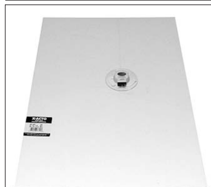
PHOTO 1: Foam-core posterboard with SoundPad exciter attached.
