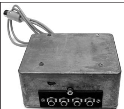
PHOTO 2: Head amp in 4" x 3" diecast box (the gray wires are the twin shielded power leads that connect with the batteries that were housed in a separate box in the prototype).
