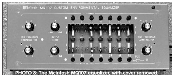
PHOTO 8: The McIntosh MQ107 equalizer, with cover removed.
