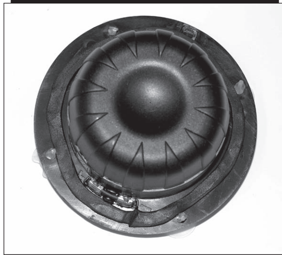
PHOTO 6: Caulk applied to driver frame.
