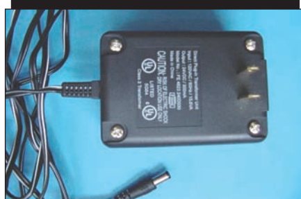
PHOTO 6: AC line “wall wart.”
