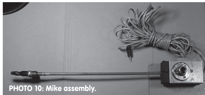
FIGURE 6: High-performance microphone. Low noise current-mirror preamp in 3\frac{1}{4}'' \times 2\frac{1}{8}'' \times 1\frac{5}{8}'' Bud Box, attached to 13'' \times \frac{1}{4}'' O.D. copper tube, "mike wand."
