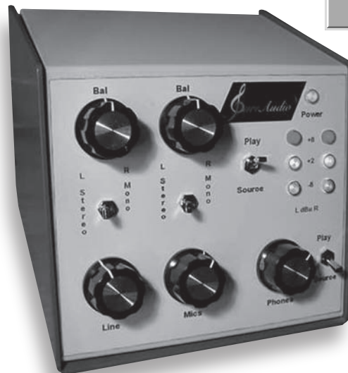
PHOTO 1: PM-2 preamp mixer/monitor.
