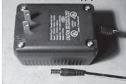
PHOTO 3: 24V DC wall supply.
