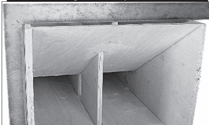
PHOTO 3: Installing the brace for plate 6.
