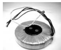
2:1 ratio Step-down Toroidal Transformer, 6.75" dia. x 1.4" Max. 240 VAC input, 250VA
