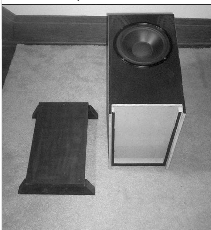
PHOTO 3: Sub with port bottom removed.
