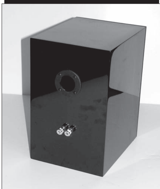
PHOTO 5: Rear of enclosure with components installed.
