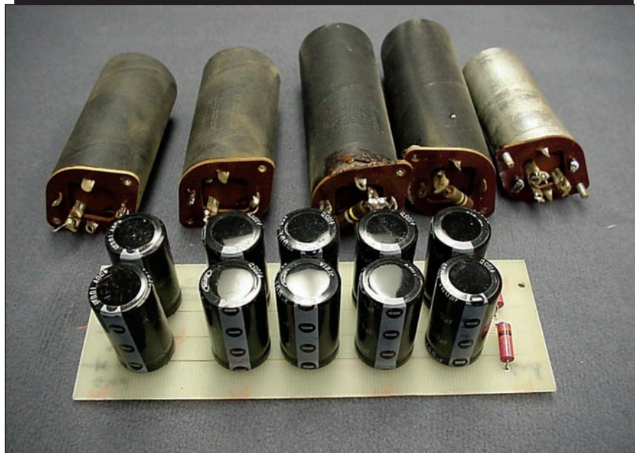
PHOTO 3: Replacing the capacitors.
