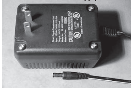
PHOTO 3: 24V DC wall supply.
