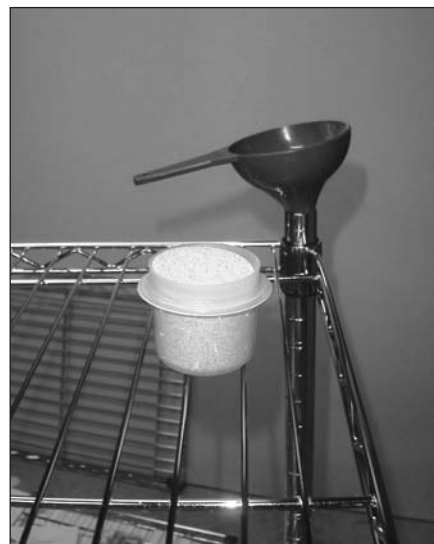
PHOTO 3: Filling shelf legs with sand.
