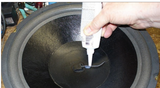
PHOTO 3: Gluing the accelerometer cable to the woofer cone.
