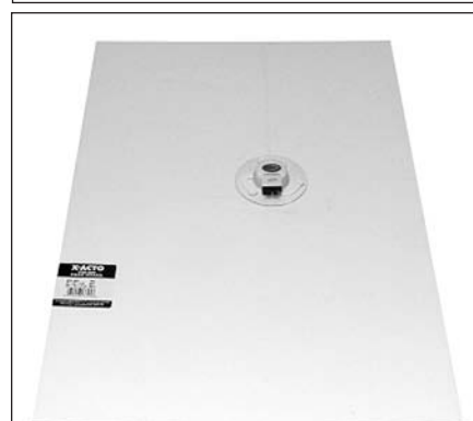
PHOTO 1: Foam-core posterboard with SoundPad exciter attached.
