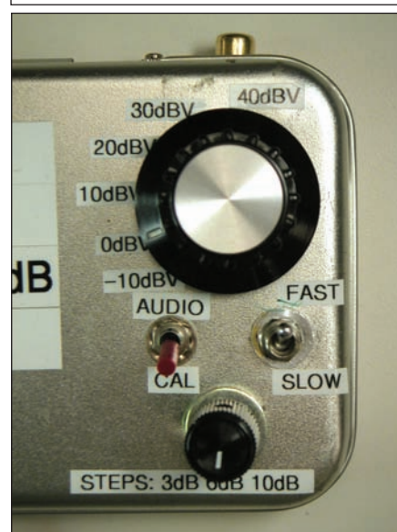
PHOTO 4: Step generator controls. a) input attenuator. b) calibration switch. c) decay: 6dB/sec or 6dB/100ms. d) dB step size. e) phono jack audio input. f) submini jack dB step output.
