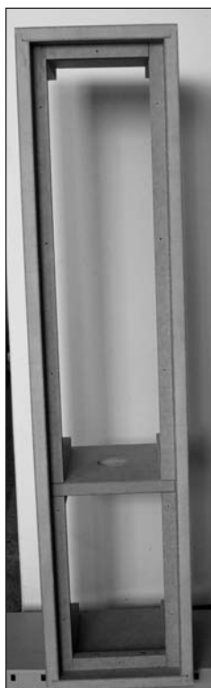
PHOTO 1: Cabinet internal frame.
