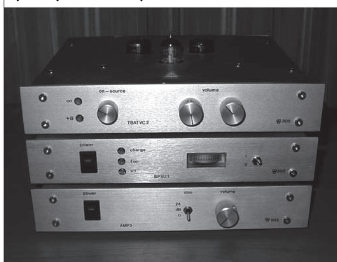
PHOTO 5: ECC86-based battery-powered preamplifier and amplifier with attenuator.
