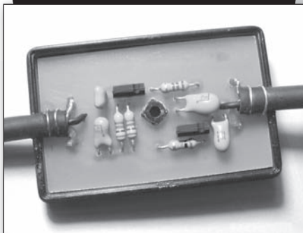
PHOTO 1: Amplifier in Radio Shack box.
