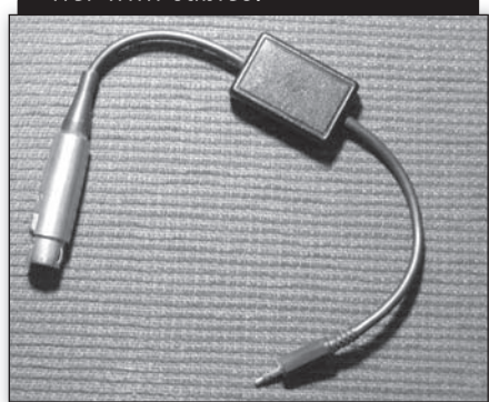
PHOTO 2: Completed amplifier with cables.
