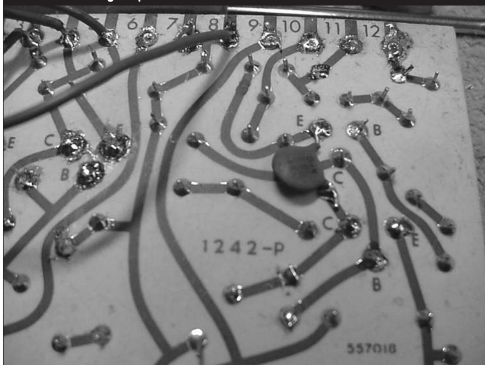
PHOTO 3: Soldering the pins on the board underside.
